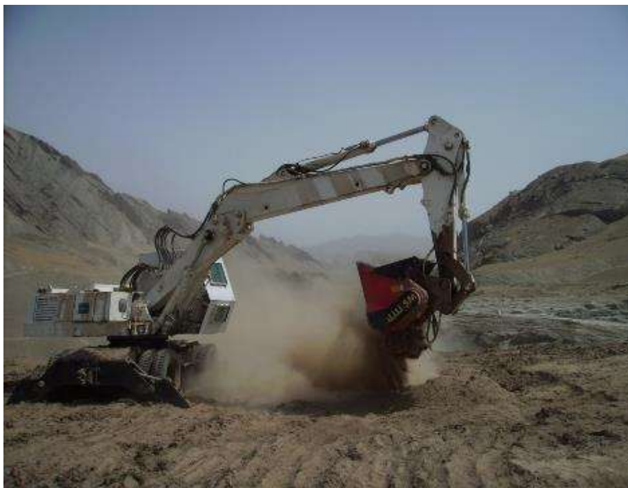
Figure 2 – Crushing bucket attached to a wheeled excavator, processing material from a spoil pile – The HALO Trust
