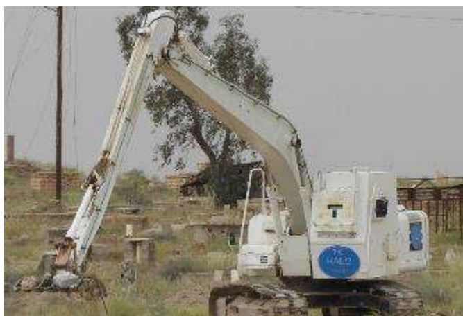
a) Tracked excavator with rake attachment – typically used for technical survey or clearance of IEDs
