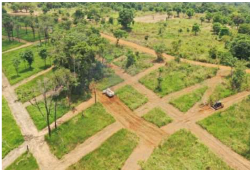
Figure 17 – Ground preparation of systematic technical survey lanes using a bespoke demining machine with tiller attachment – Norwegian Peoples Aid
