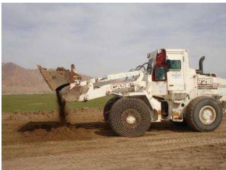
Figure 11 – Soil passed through the filter and out of the bottom of the bucket – The HALO Trust
