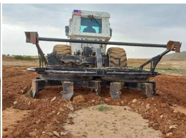
b) Rotary mine comb (RMC) attached to a tractor – typically used for clearance of minimum metal AV mines
