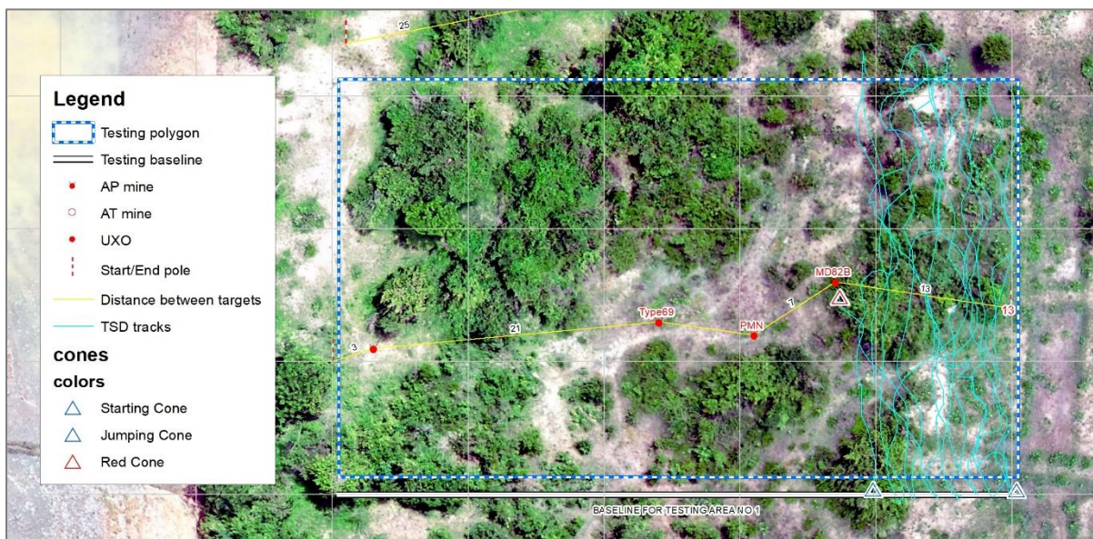
Figure 4: TSD testing box 30x50 meters wide
