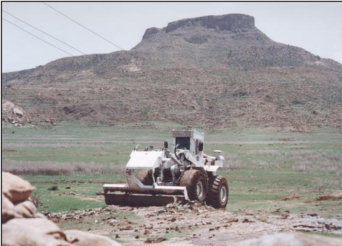
A Pearson Roller attached to a CASE front-end loader working near Senafe, Eritrea.
