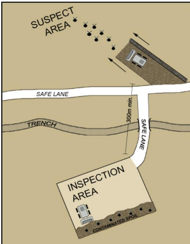
Fig 6: Suggested positioning of inspection area in relation to suspect area for armoured bucket mine clearance.
