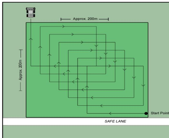
Fig. 1: Section of a piece of land in a suspect area (approx. 200m x 200m). 1<sup>st</sup> phase of rolling in concentric box pattern in area where mines are not expected. Pattern is optional but this technique has been proven effective
