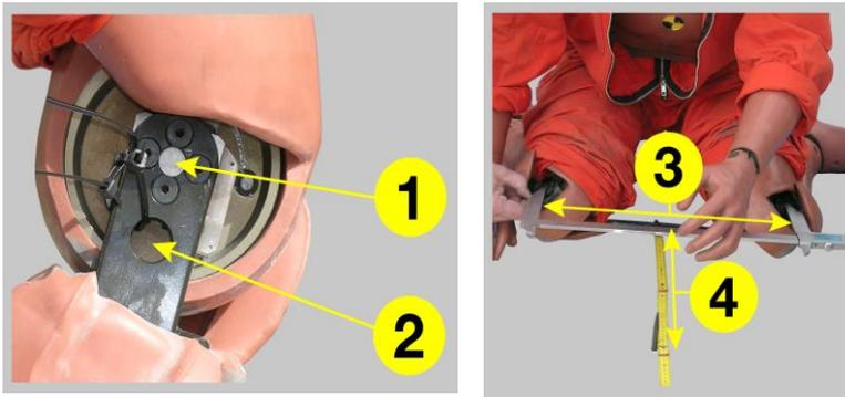
Key: 1 = Pivot point of knee joint      3 = 400 mm (measured from the outside of the pivot point of knee joint)
