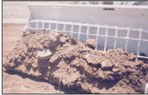
HALO has adapted armoured buckets with a gill to separate AT mines from soil and AP mines for use in areas where the occasional AT mine may exist.
